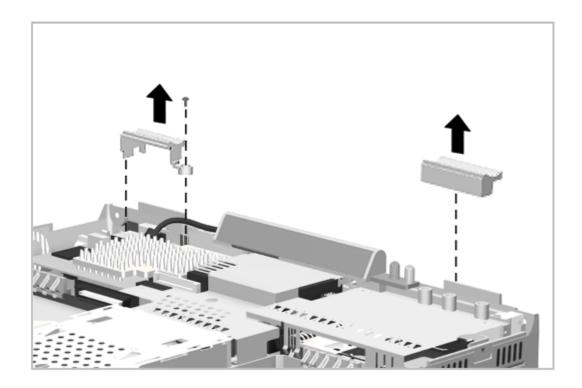
Figure 5-36. Removing the Clutch Cradles
